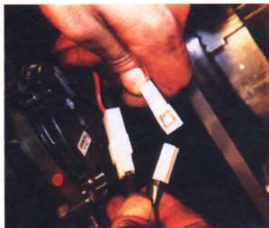
12. After the electrical wires were sized and cut, the ends were stripped and the connectors were crimped and connected.
