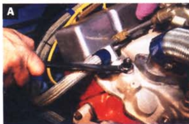
10. A&B A 3/8-inch-diameter pipe thread tap was used to thread the SPAL thermostat sending unit hole.
