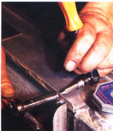
7. The upper and lower mounting brackets were aligned and matted with the side mounting brackets, then secured.
