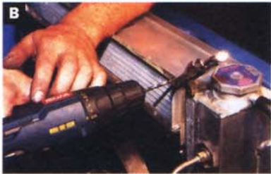
6. A&B With the side mounting brackets mounted onto the SPAL Dual Fan unit, Chris lowered and aligned everything, then temporarily secured the unit to the Fluidyne radiator core frame with vise grips. With the SPAL Dual Fan unit aligned and secured, it was then drilled.
