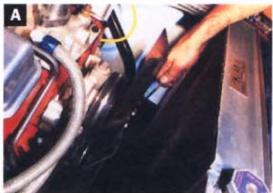
2. A&B After removing the fan shroud, Chris used a 1/2-inch wrench to remove the Flex-a-lite fan.
