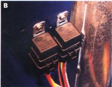
8. A&B The SPAL Dual Fan relay switches were mounted on the lower portion of the fenderwell.
