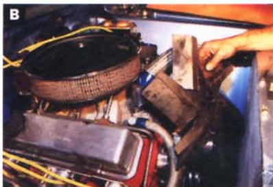
2. A&B After removing the fan shroud, Chris used a 1/2-inch wrench to remove the Flex-a-lite fan.
