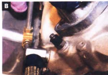
11. A&B The thermostat sending unit was then secured.
