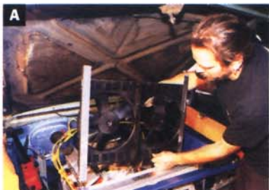
5. A&B The custom-fabricated side mounting brackets were notched and drilled, then mounted to the SPAL Dual Fan shroud.
