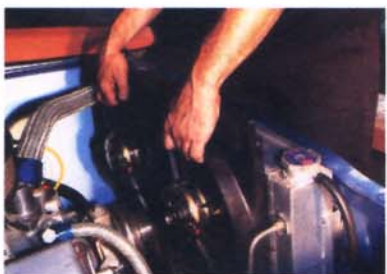
3. The SPAL Dual Fan unit was lowered for a test fit to determine the mounting locations.
