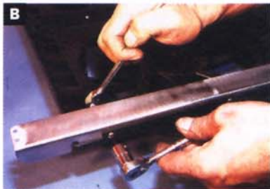
5. A&B The custom-fabricated side mounting brackets were notched and drilled, then mounted to the SPAL Dual Fan shroud.
