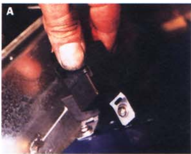
7. The upper and lower mounting brackets were aligned and matted with the side mounting brackets, then secured.
