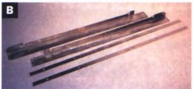
4. A,B&C Chris fabricated four mounting brackets to secure the Dual Fan unit on the Fluidyne frame supports, rather than pierce through the aluminum radiator core.
