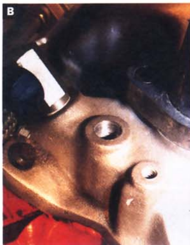
10. A&B A 3/8-inch-diameter pipe thread tap was used to thread the SPAL thermostat sending unit hole.
