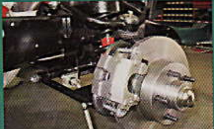
33. This rear photo of the front TCI disc brake assembly exposes the new TCI two-piston caliper.
