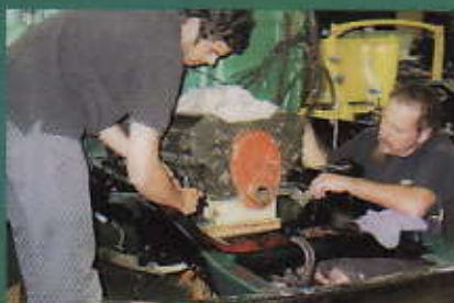
22. After the engine mount welds had cooled, Brian and Chris removed the engine mount bolts.
