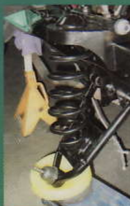
26. A floor jack was used to assist in installing the TCI coil spring.
