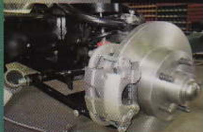
25. A long Grade-8 bolt was inserted into the lower A-arm mounting brackets and on the A-arm, then they were secured.
