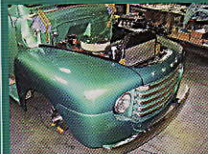
35. After the front sheetmetal was aligned, it was mounted at the mounting points of the frame and firewall.
