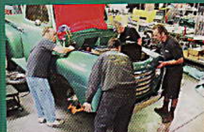
34. How many guys does it take to mount the front sheetmetal on a '49 F-1? Four, one on each corner.
