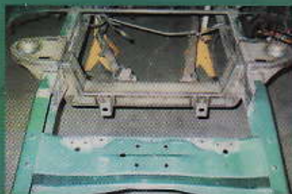
18. The stout TCI crossmember and shock towers were TIG-welded in place between the framerrails.
