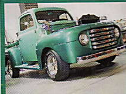
38. Replacing the original Ford F-1 straight axle/leaf spring front suspension with TCI's IFS has slightly dropped the nose, creating a slight rake and just what the customer wanted.
