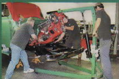
22. After the engine mount welds had cooled, Brian and Chris removed the engine mount bolts.
