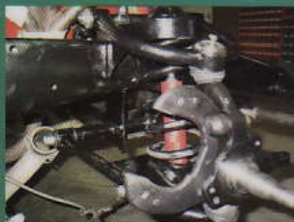
28. For this application, the customer wanted to maintain the stock ride height but achieve the ride quality of the IFS (independent front suspension).
