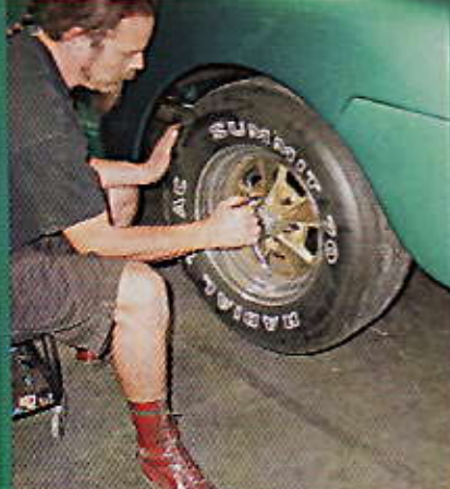
37. With the TCI IFS kit installed, Chris remounted the front wheels and tires.
