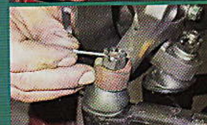
31. A&B After threading the steering rod end to the tie rod, it was then aligned and secured with a castle nut and cotter pin.
