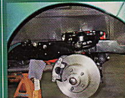
36. Peering through the front wheelwell, we could see the final TCI front IFS conversion complete.
