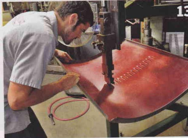
> The centerline row of louvers is the shortest because of the handle that will be installed later. The laser light is a big help to the louvers straight and in the middle of the scribed centerline.
