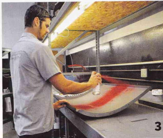
3 > To make the lines easier to see, Brian used marking paint on the inside of the lid.
