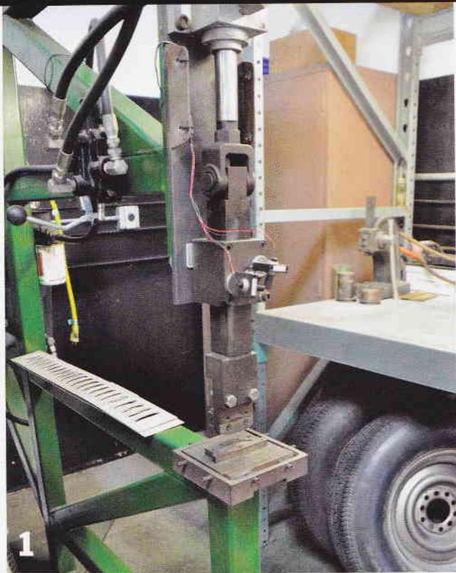
1 > The louver machine at Wheeler's Speed Shop is the usual type, but Brian Wheeler has installed two lasers to make it a lot easier to get the louvers nice and straight.
