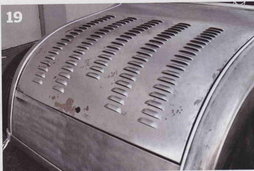
> We wanted to see how the louvered decklid would look on the car, so the skin was installed on the decklid and then installed on the roadster.
