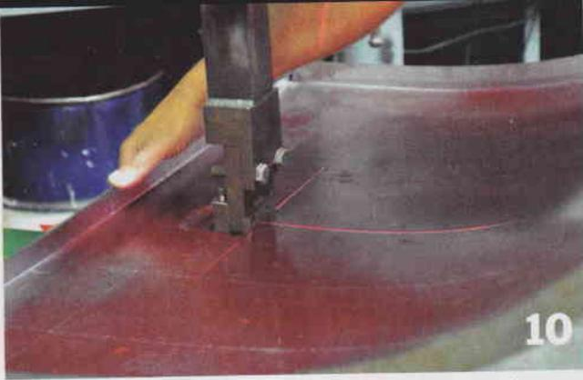
> When the first and second louvers are stamped, the tool uses the previous louver for lining up the next louver to be stamped.
